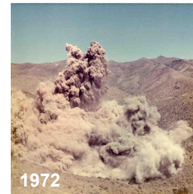
Old Reliable - Largest non-nuclear explosion in the US (1972), in-situ leaching of copper by Ranchers Exploration
