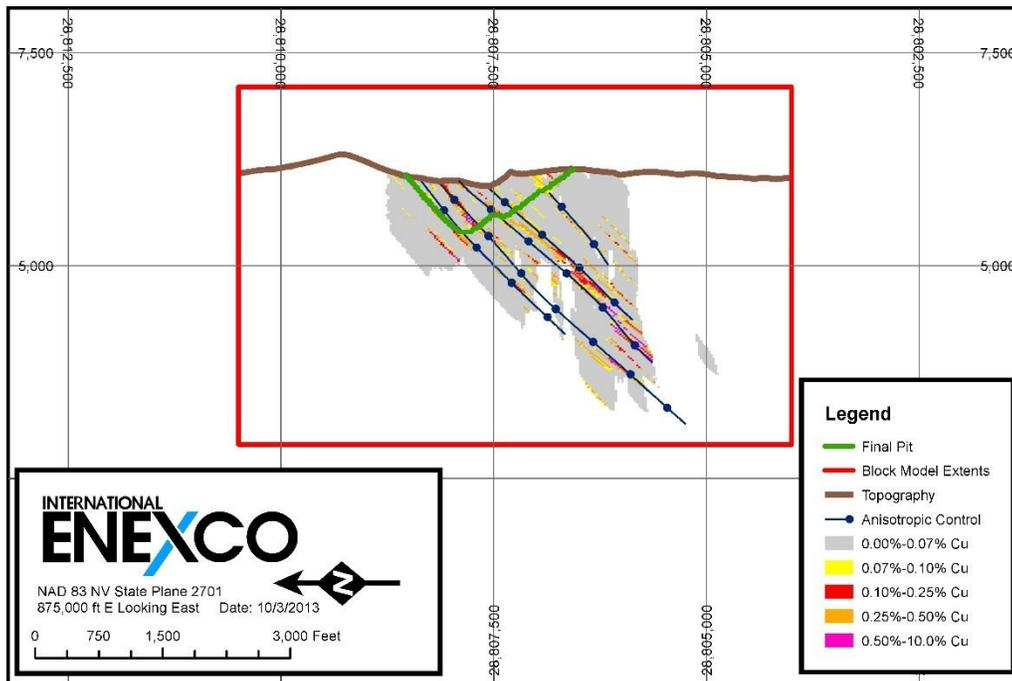
**Figure 14-9 28,807,800 North, West-East Section through Block Model**
